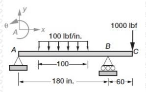
(b) Find also the Bending Moment diagram of the beam given below
